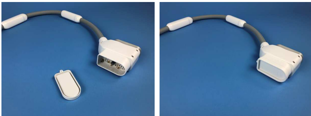
Figure 14: Attach cover onto coil connector of the Endorectal Coil.
